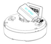
1. From back of heat alarm, remove the mounting plate by turning it counterclockwise.
